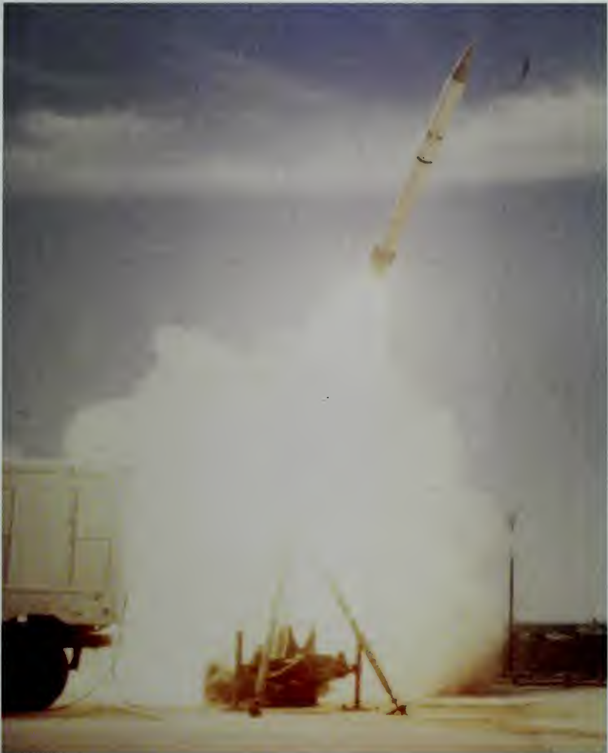
Fig. 3-12. Guided by 216 attitude control motors, the Flexible Lightweight Agile Guided Experiment demonstrated the feasibility of kinetic energy intercepts at short ranges.
